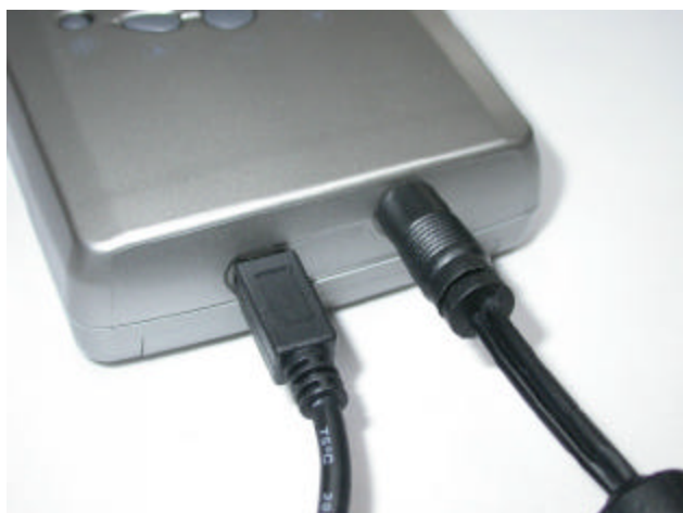
USB 2.0 cable and DC Power connected
